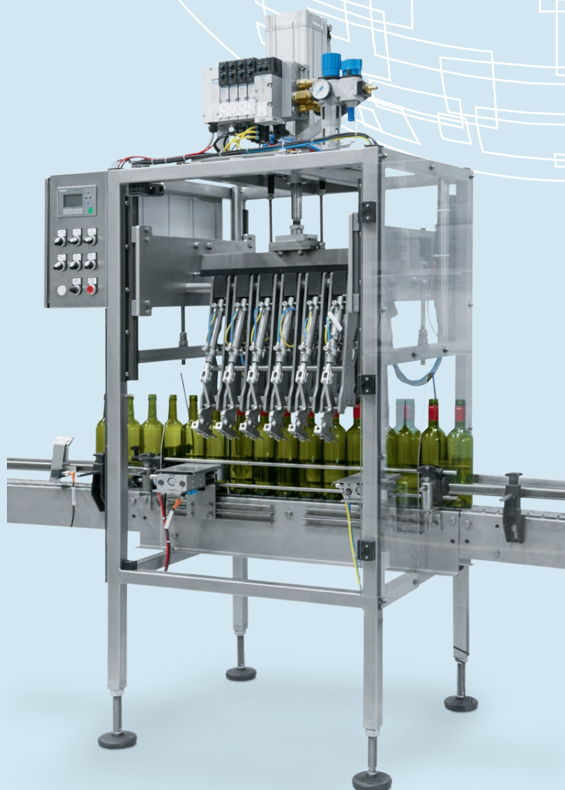
Compact design: the pneumatic neck foil remover with valve terminal VTSA.
